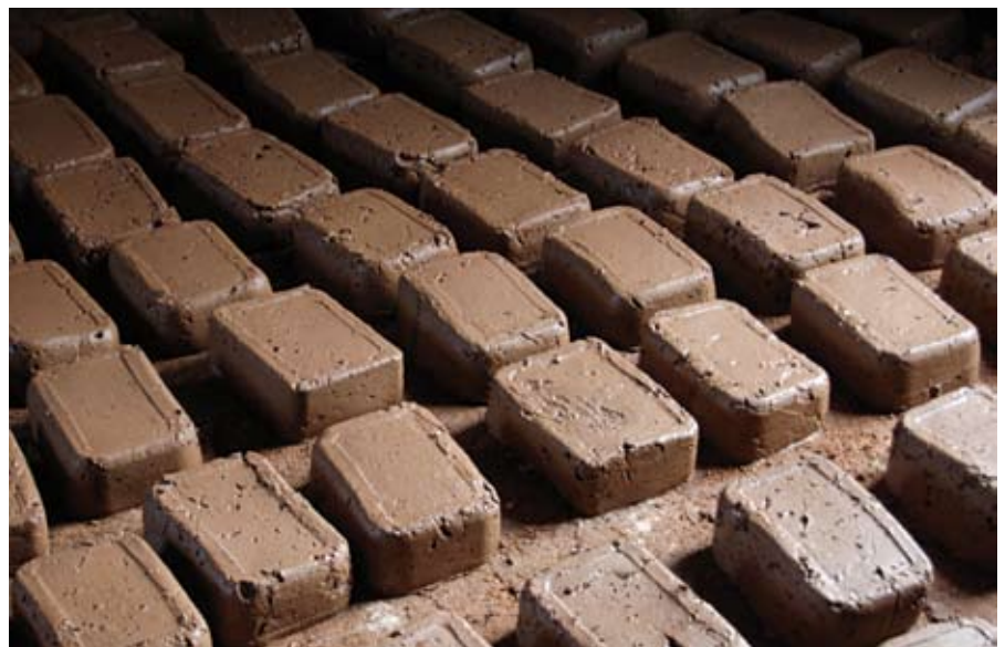
Sun-dried clay bricks were used for sections of walls that required extra strength
